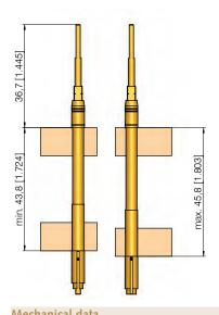
The VF 5 is mounted in the KS-VF5 030 which is pressed into a second plate to fix the receptacle securely and prevent rotation. The distance between the plates is 44.8 m
